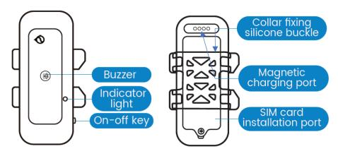
By looking at the status indicator, you can understand the working condition of the device. The status of the indicator is as follows:
